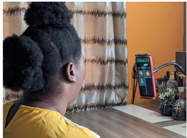
Figure 4: P4 operating the Look to Speak application while sitting on her wheelchair, showing good alignment between the position of the eyes and the camera
