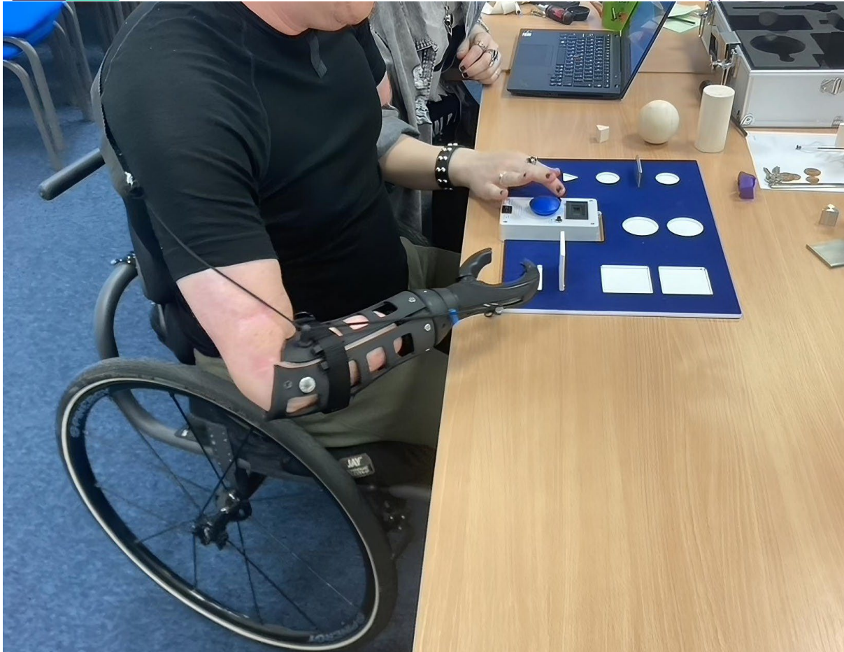
Figure 6. Participant E using the 3D printed socket and voluntary-closing prehensor during the lateral grasping task of the SHAP test.
