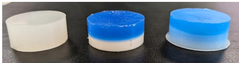
Figure 1: Representative examples of samples for compression testing: Ecoflex 00-30 (left), moulded composite (middle) of Ecoflex 00-10 (blue) and Ecoflex 00-30 (white), and printed composite (right) of Ecoflex 00-10 (blue) and Ecoflex 00-30 (white).
