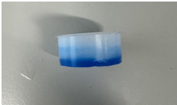
Figure 3: A composite graded print with Ecoflex 10 and Ecoflex 30
