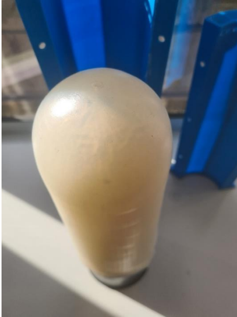
Figure 18: A repaired liner using a novel remoulding technique
