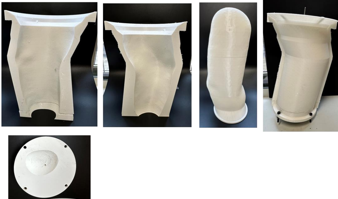
Figure 6: Custom mould sections for an upper residual limb
