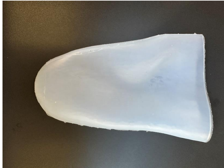
Figure 16: Inner silicone layer for custom liner. Testing of fabric layer construction will now proceed
