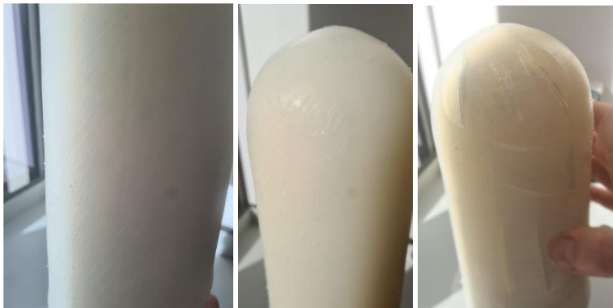
Figure 7: Damage applied to liner to simulate use
