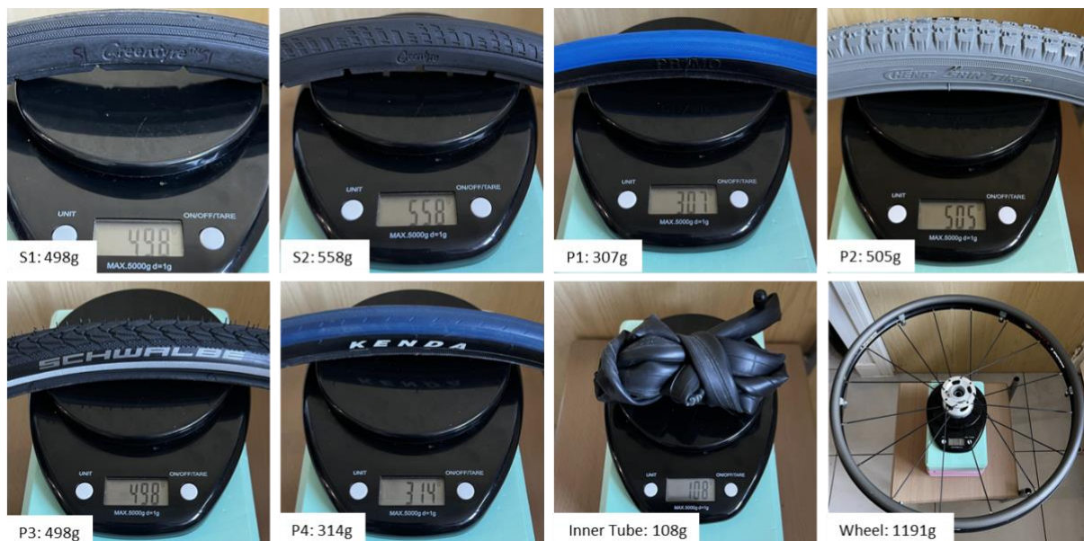
Figure 3 - Images of wheelchair tyres (S=Solid, P=Pneumatic), pneumatic tyre inner tube, and Fusion 16 spoke wheel used for testing. Mass is also shown in grams.
