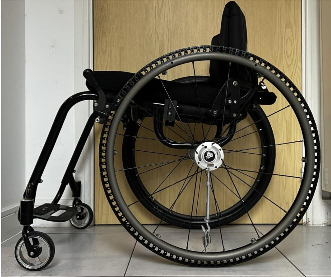
Figure 13 - The first wheelchair FS-NPT mounted onto an active wheelchair (RGK Hi-Lite Titanium)
